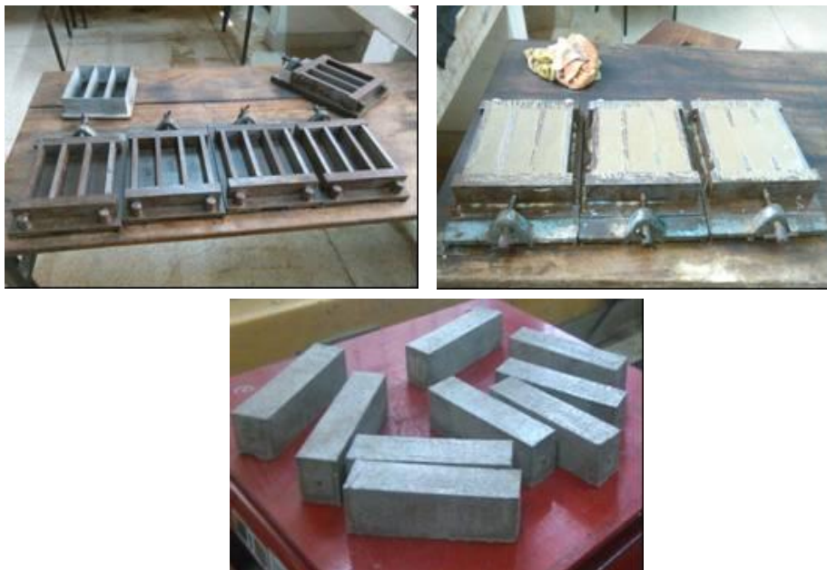
Figure 4. Moulds – top left, samples after casting (right –top), and mortar prisms (bottom)
