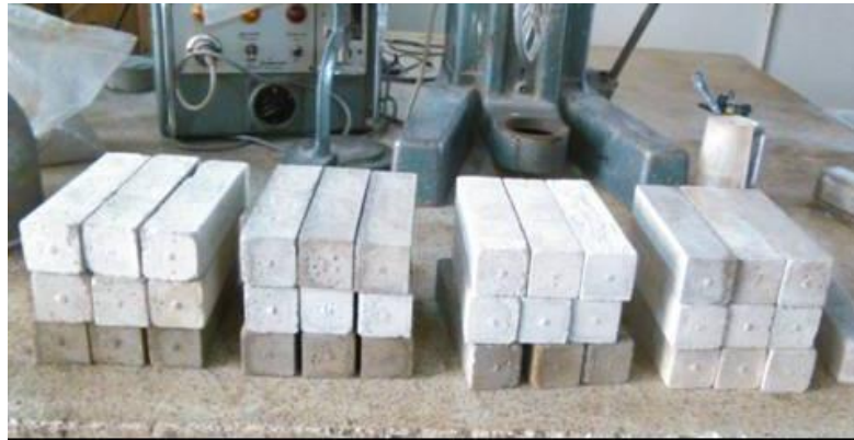
Figure 11. Prism specimens after Water Absorption test.
