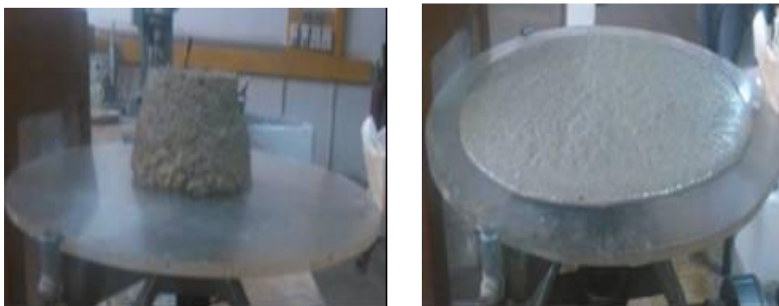
Figure 2. Flow table test as conducted at UDSM Building Materials Laboratory
