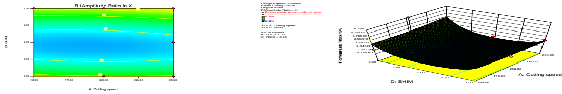
Figure 6. Contour and 3D plots for AD DOC 1.2-mm Feed 0.05 mm/tooth at R1 Amplitude Ratio in X
