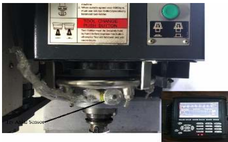
Figure 1 VMC milling machine with CoCo80 Dynamic Signal analyzer with Try Axial Sensor
