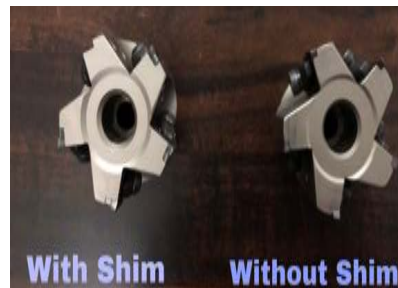
Figure 2 face milling tool 63 mm dia with shim and without shim face mill
