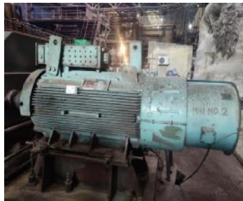
Fig.3. Sensor installed for condition monitoring on induction motor
