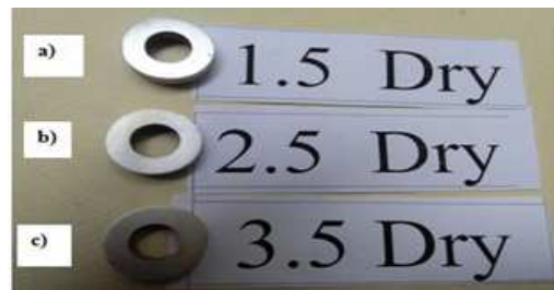
Fig.2 Photographs of ring specimens with: a) 1.5 μm surface roughness value, b) 2.5 μm surface roughness value and c) 3.5 μm surface roughness value.
