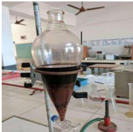
Figure 2. Separation of Glycerol and Esters
