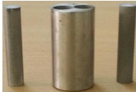
Figure 1. Wear Specimen machined by EDM
