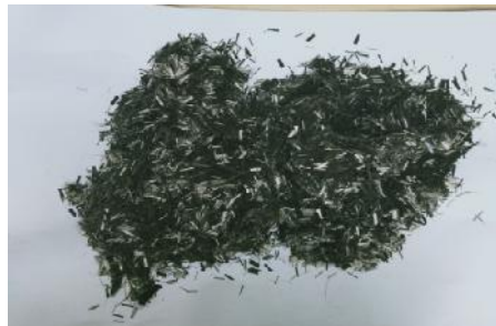
Figure 1 Chopped carbon fiber
