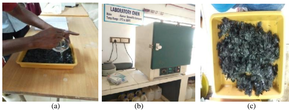
Figure 3(a-c) Steps involved in HNO 3 chemical treatment on CF
