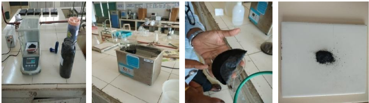
Figure 5. Sequential operations carried out in MWCNT surface oxidation to form MWCNT-F
