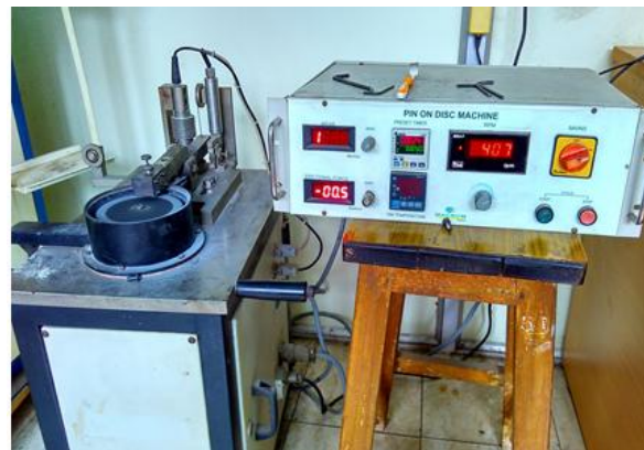
Figure 1. Experimental set up of pin-on-disc wear tester.
