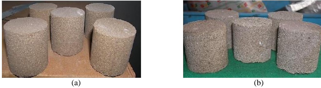
Figure 2: Shows the standard samples of: (a) 100% Silica Sand (b) 100% GBF Slag and
