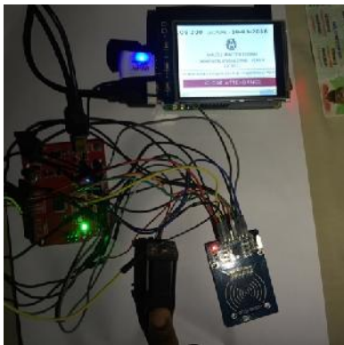
After a student taps the RFID reader, his details are displayed on the touchscreen with a notification to take a scan of his fingerprint. The fingerprint reader lights up –to wait for a fingerprint style.
