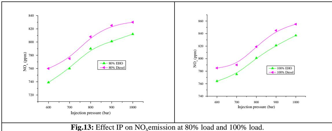
Fig.13: Effect IP on NO<sub>x</sub>emission at 80% load and 100% load.
