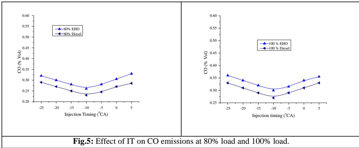
Fig.5: Effect of IT on CO emissions at 80% load and 100% load.
