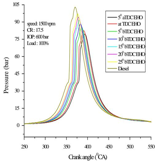
**Fig. 8:** Effect of IT on Peak Pressure at 100% load.
