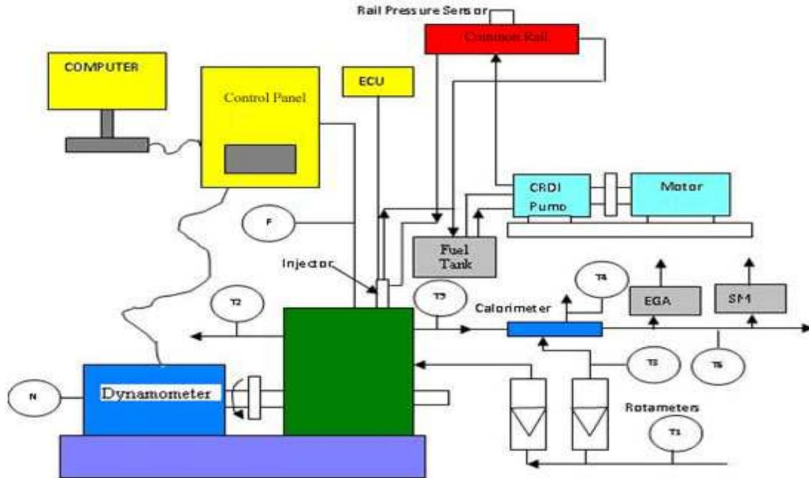
T1, T3 – Inlet Water Temperature, T2 – Outlet Engine Jacket Water Temperature
