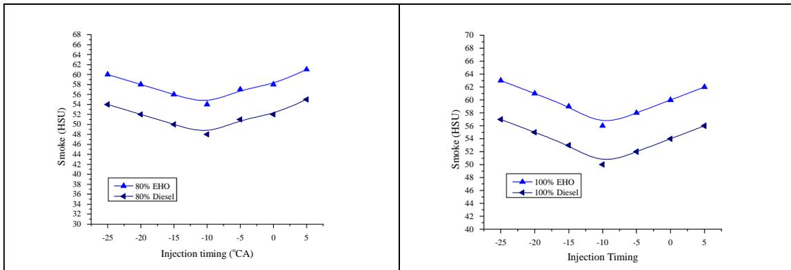
**Fig. 7:** Effect of IT on Smoke at 80% load and 100% load.
