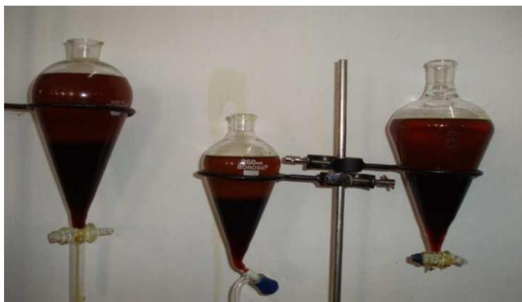
Fig. 1. Biodiesel separation flask
