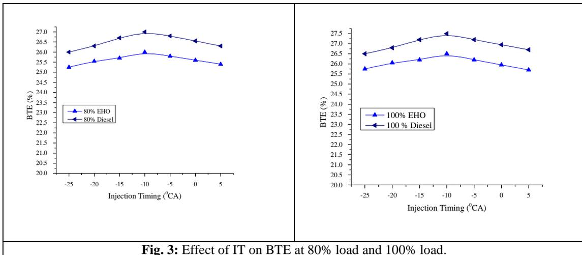
Fig. 3: Effect of IT on BTE at 80% load and 100% load.
