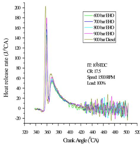
**Fig. 16:** Effect of IP on HRR at 100% load.
