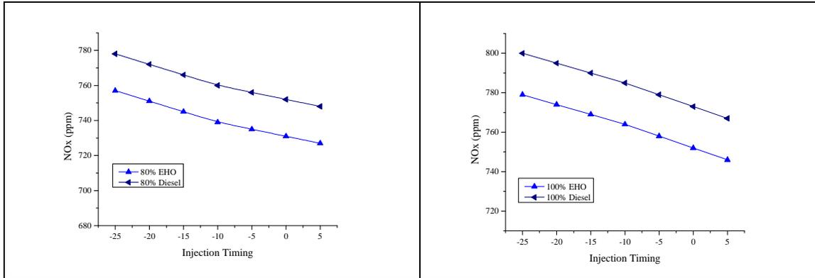
**Fig. 6:** Effect of IT on NO<sub>x</sub> at 80% load and 100% load.
