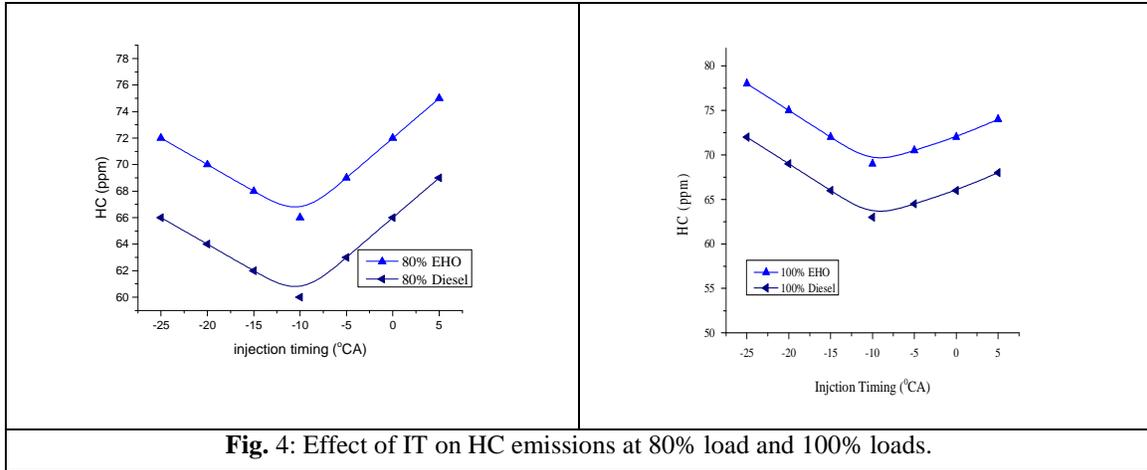
Fig. 4: Effect of IT on HC emissions at 80% load and 100% loads.
