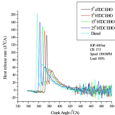
**Fig. 9:** Effect of IT on HRR at 100% load.
