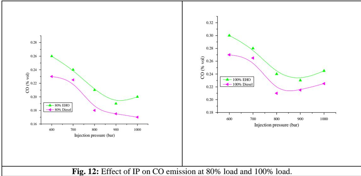
Fig. 12: Effect of IP on CO emission at 80% load and 100% load.
