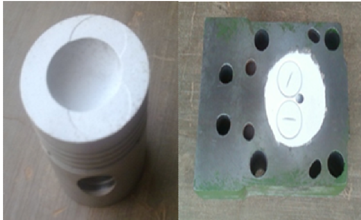
Piston coated with \text{Al}_2\text{O}_3 Cylinder head coated with \text{Al}_2\text{O}_3 Figure5. \text{Al}_2\text{O}_3 coated piston and cylinder head
