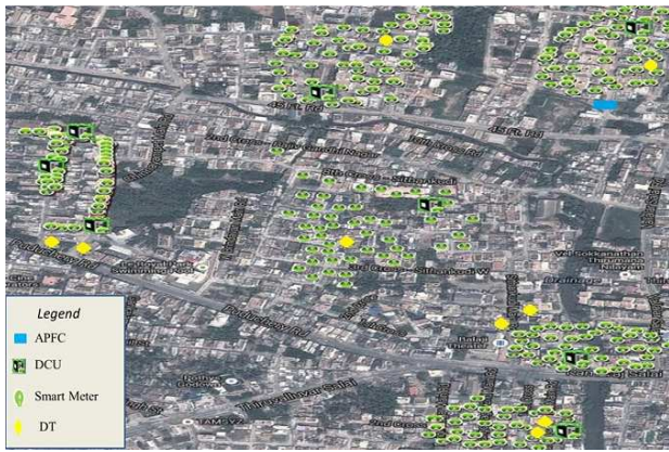
Figure 4, GPS location of Smart meters, DCU and Distribution Transformer
