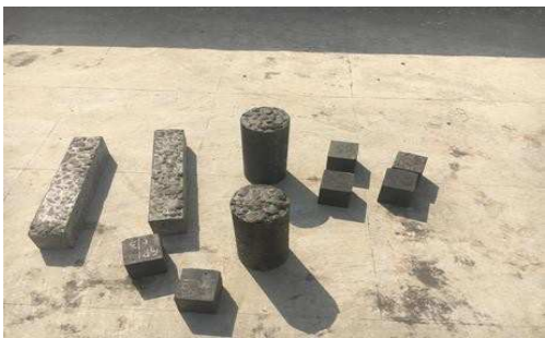
Figure 10. Blocks kept under sunlight for curing
