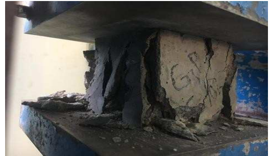
Figure 11. Failure of the cube
