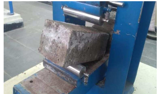
Figure 12. Failure of the beam
