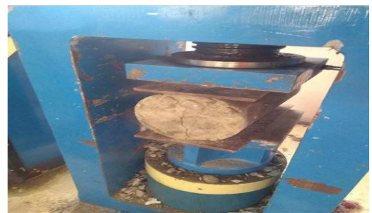
Figure 13. Failure of cylinder
