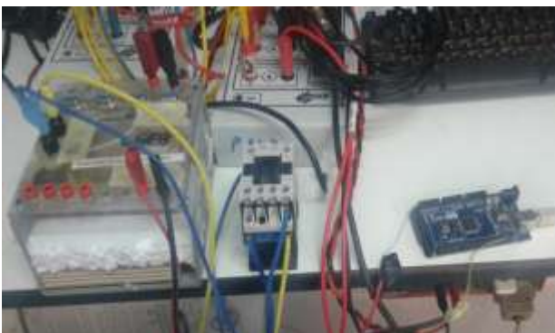
Figure 3. Circuit to control the time of the ITSC fault by 'Arduino card'
