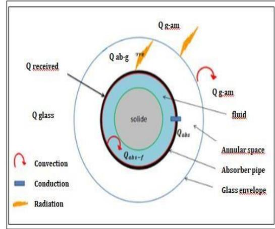
Figure 1. Different heat transfer modes
