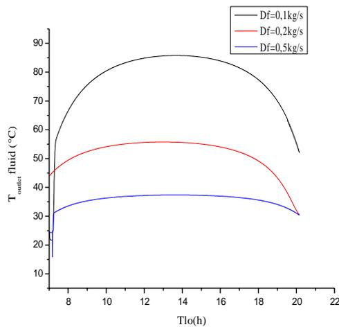
Figure 6. Variation of the outlet Fluid Temperature for different mass flow rate
