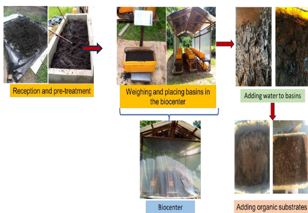
Figure 6 : Landfarming method adopted (pre-treatment of polluted sludge and installation of basins in the bio-center)
