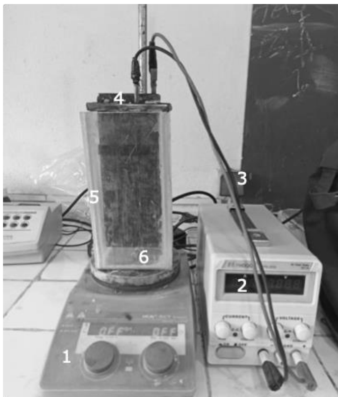
Figure 1: Experimental Set-up for Electrocoagulation. (1) magnetic stirrer, (2) DC power supply, (3) wires, (4) electrode, (5) Electrocoagulation cell, (6) magnetic stirrer bar.
