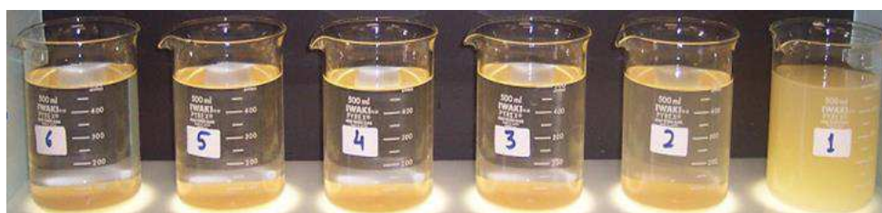
Figure 3: Standard Jar test setup for coagulation of turbid water with seed extracts. Concentration ranges 1 to 6 in the order 0, 20, 40, 60, 80 and 100 mg/l respectively.
