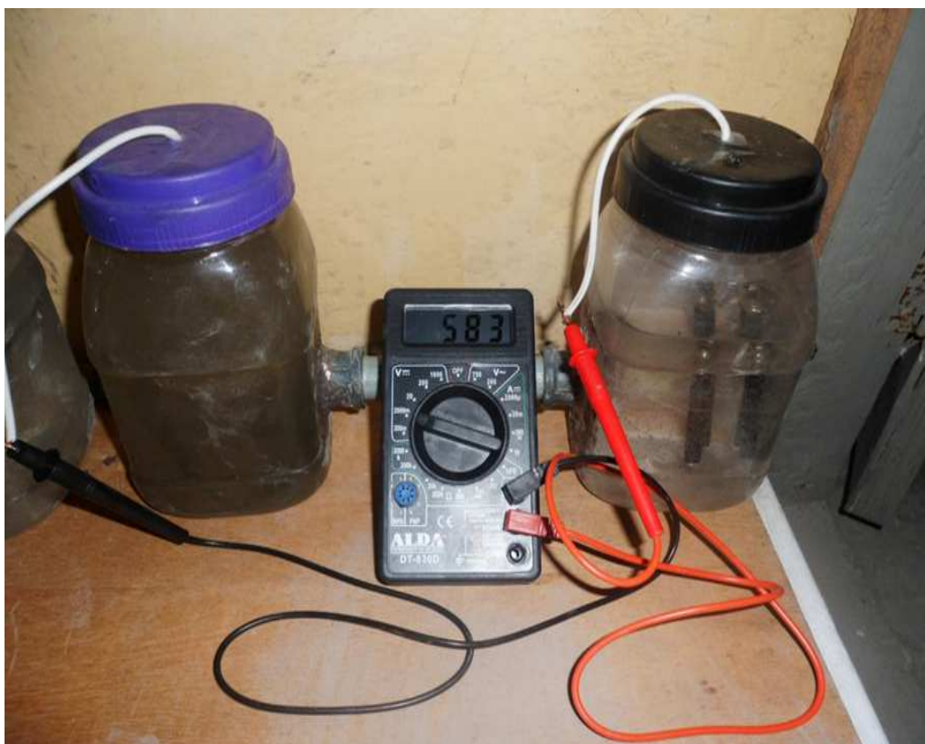
Figure 1: A complete set up of a H-type microbial fuel cell using carbon electrodes.
