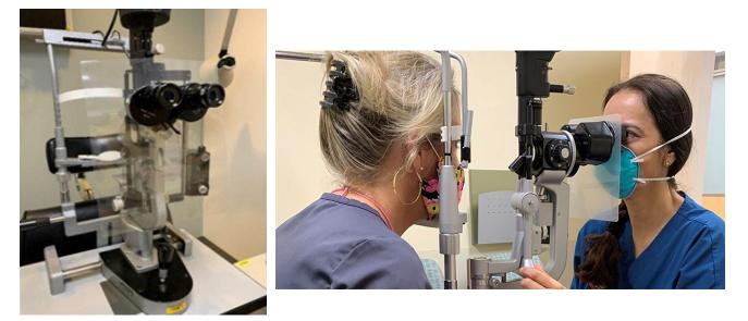
A slit-lamp shield to protect the examiner as designed by Moran Technicians Stein Erickson, Emily Petersen and Anna Reed together with help from others: made by passing two lamination sheets together through a laminator without anything in-between. Results in a rigid shield which can be cleaned with alcohol and reused. Other materials that may be used include used X-Ray films but these do not have the clarity needed.
