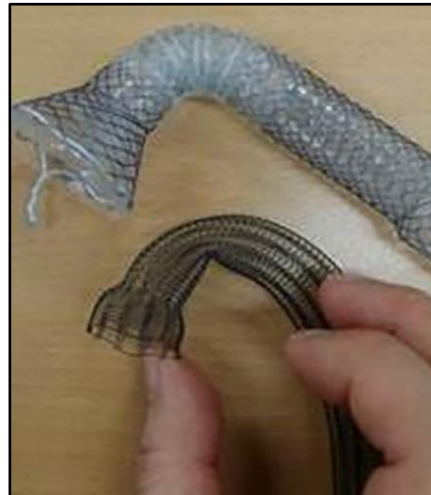
Figure 4 Flexible neck maintains pliability
