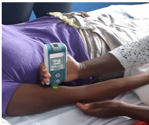
Figure 1 MyotonPRO device in use for assessing the mechanical properties of the Biceps Brachii muscle.
