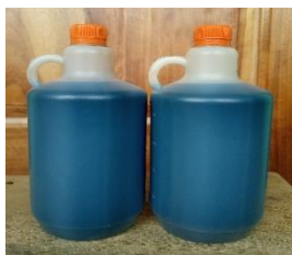
Fig. 5 Samples of Liquid Fuel obtained from the Pyrolysis of End-of-Life Vehicle Tyres
