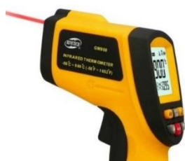
Fig. 3 BENETECH GM900 Infrared Thermometer used for Temperature Measurements in this Investigation
