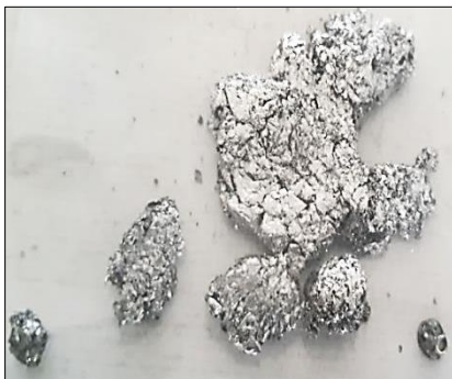
Fig. 4 Sample of Silver Metal Electrodeposited at the Cathode at an applied Potential of 1.8 V
