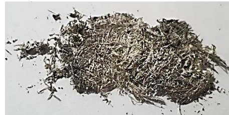
Fig. 5 Illustration of Dendrite Formation and Anode Degradation at High Current Densities and Applied Potential of 2.5 V
