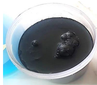
Fig. 20 Change in Colour of the Silver Nitrate Electrolyte to Black at Applied Potential of 2.5 V
