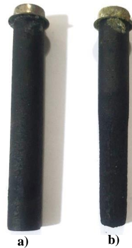
Fig. 19 Nature of Graphite Anode after Electrowinning at Applied Potential of a) 1.5 V and b) 2.5 V
