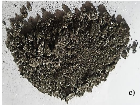
Fig. 6 Nature of Silver Metal Electrodeposited at the Cathode at an applied Potential of a) 1.2 V, b) 1.5 V and c) 2.0 V
