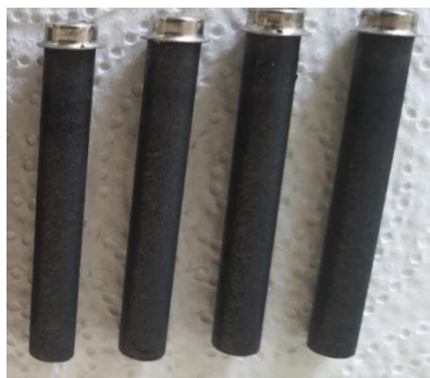
Fig. 1 Samples of Graphite Rods recovered from Spent Zinc Carbon Batteries
