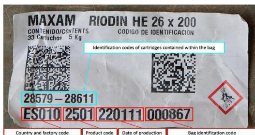
Fig. 11 :Sample of Labelling of Explosives with Traceability Number
