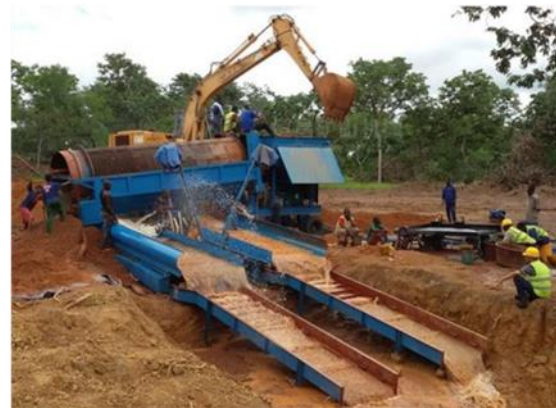
Fig. 4 Alluvial Washing Plant Method (Source: Anon., 2015)
