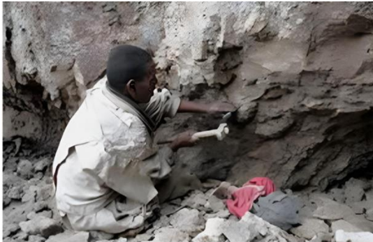
Fig. 5 Chisel and Hammer Method (Source: Anon., 2009)
