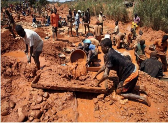
Fig. 3 Dig and Wash Mining Method (Source: Anon., 2009) “More blade” method
