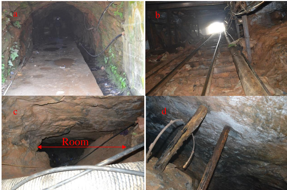
Fig.s 9 (a) An Adit at the Mine, (b) The Mine Shaft with Rails, (c) The Room and Pillar Mining Method, (d) Timber Supports Underground at Mohammed and Brothers Mine
