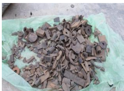
Fig. 2 48-h air-dried, shredded waste vehicle tyres Feedstock
