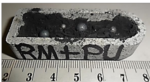
Fig. 12 Droplets of Metallic Iron obtained after Reduction of Fe_2O_3 -PU Composite at 1550 °C
