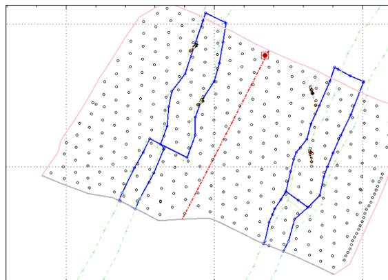
**Fig. 8 Plan View of BMM® Balls in Drill Holes**
