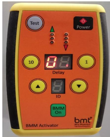
**Fig. 4 Blast Movement Monitor (BMM®) Ball Activator** (Anon., 2015)
