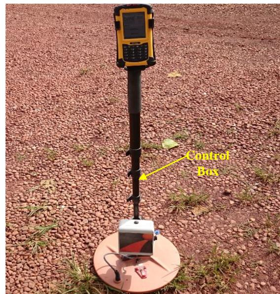
**Fig. 5 Blast Movement Monitor (BMM®) Ball Detector** (Anon., 2015)
