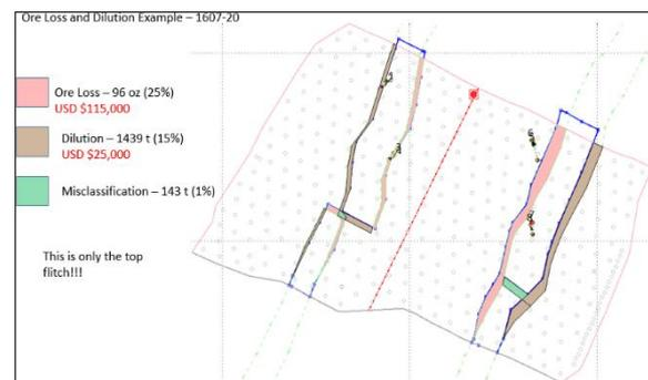
Fig. 14 Calculation of Ore Loss, Dilution and Misclassification using BMM Explorer
