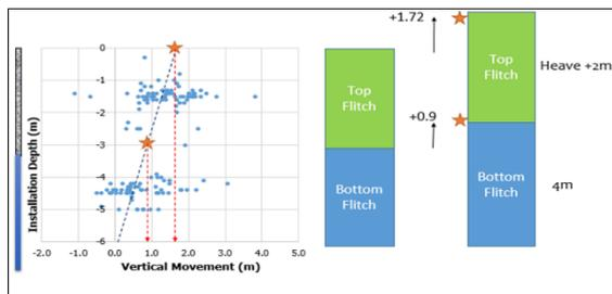
Fig. 11 Vertical Movement Interpretation (not drawn to scale)
