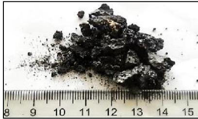
Fig. 8 Material Produced after Reduction of Mn 3 O 4 by Postconsumer PP
