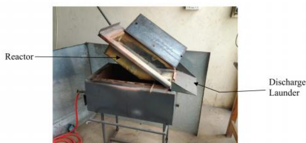
Fig. 1(c) Reactor Lifted for Discharging of Carbonaceous Products
