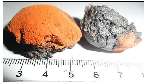
Fig. 20 Extremely Sintered Bauxite-Polymer Composite
