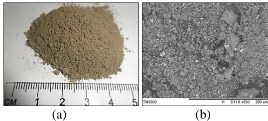
Fig. 13 (a) Photograph and (b) SEM Photomicrograph of Magnetic Fraction obtained after Heating Awaso Bauxite Ore with PWS
