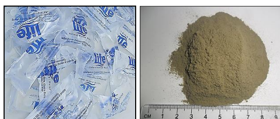
Fig 2 (a) Waste Pure Water Sachets (b) Pulverised Carbonaceous Material obtained after Heat Treatment of Waste Pure Water Sachets
