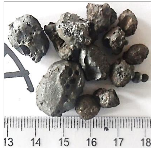
Fig. 8 Samples of Reduced Metal obtained after Reduction of Maximum Blend of 15% Ankerite Ore
