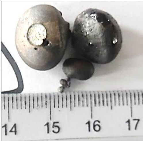
Fig. 9 Samples of Reduced Metal obtained after Reduction of Blend Consisting of 50% Ankerite Ore
