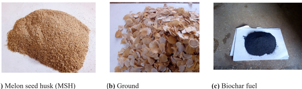
Fig 1: Morphological changes of melon seed biomass during pyrolysis process.
