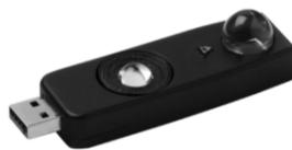
Fig. 4. LiFiNET modem (Source: Photo taken by the authors).
