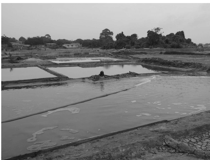
PLATE 2 Salt pan being fed with brine from dug out well
