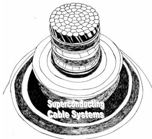
Fig. 3: Symmetric view of superconductor cable design (Nexans, 2010)
