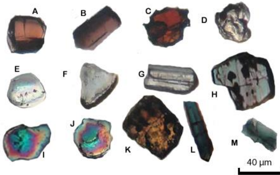
Figure 5. Some individual heavy mineral species selected under high magnification in plane polarized light (NB: A-B = Tourmaline; D = Garnet; E-F = Apatite; G-H = Zircon; I-J = Epidote; C, K = Staurolite; L-M = Zircon)
