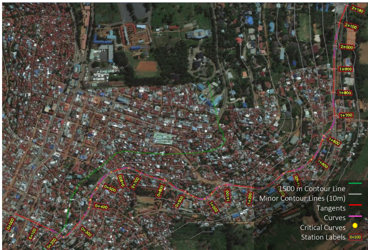
Figure 4: Road alignment plan view and station visualization. Chainage length is from 0 to 2.18Km.
