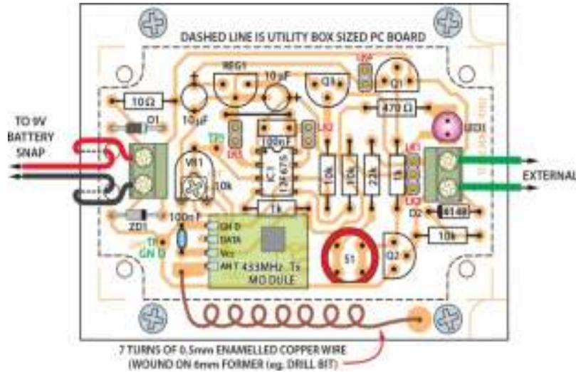
Figure 3: Overlay Diagram for the Transmitter ( Multism)
