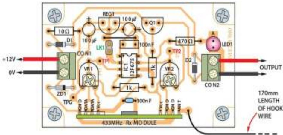
Figure 4: Overlay Diagram for the Receiver (Multism)
