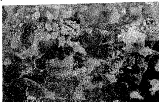
Fig. 8 The SEM micrograph of \gamma - \text{Al}_2\text{O}_3 prepared from \text{Al}(\text{acac})_3 in the presence of water at 800^\circ\text{C} by sol-gel method.
