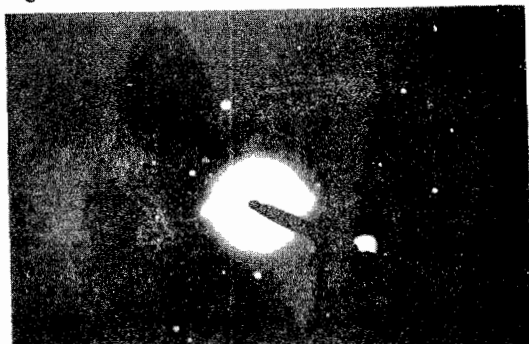
Fig. 7 The ED pattern of \alpha - \text{Al}_2\text{O}_3 prepared from \text{Al}(\text{acac})_3 at 900^\circ\text{C} by sol-gel method
