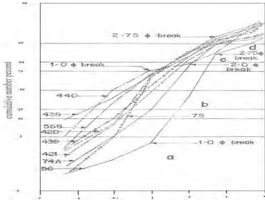
**Figure 5 :** Grain size distribution curves of the Agbani Sandstone illustrating the truncation of the curves into traction load (a), saltation load (b & c), suspension load (d)
