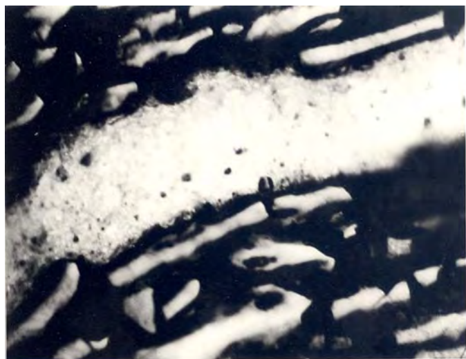
Figure 12: Massive calcite surrounded by ruptured fusinite (Reflected/oil immersion x 958)
