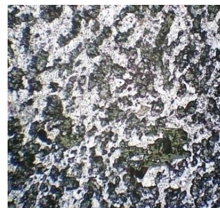
Fig: 11 Photomicrograph of meladorite (Field of view x4): showing textural interrelationships of the various minerals occurring in the meladorite of Oban Massif area.
