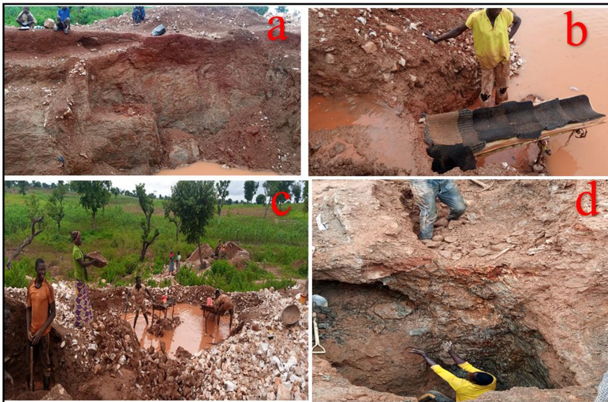
Figure 5: Panning of soils to concentrate gold grains (a-d). Pits and trenches where samples are taken sometimes up to 3m (a & d); employment of rudimentary tools (b & c) by indigenes to pan for gold using a shaking table.
