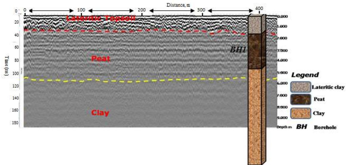
Figure 5b: GPR section of traverse 1 corroborated by borehole section BH1
