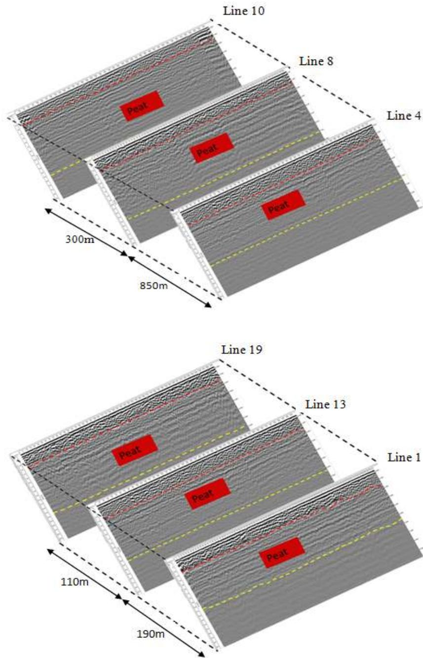
Figure 8: (a) Fence plot of the interpreted radar sections for parallel traverses 4, 8, and 10 within the study area (b) Fence plot of the interpreted radar sections for parallel traverses 1, 13, and 19 within the study area
