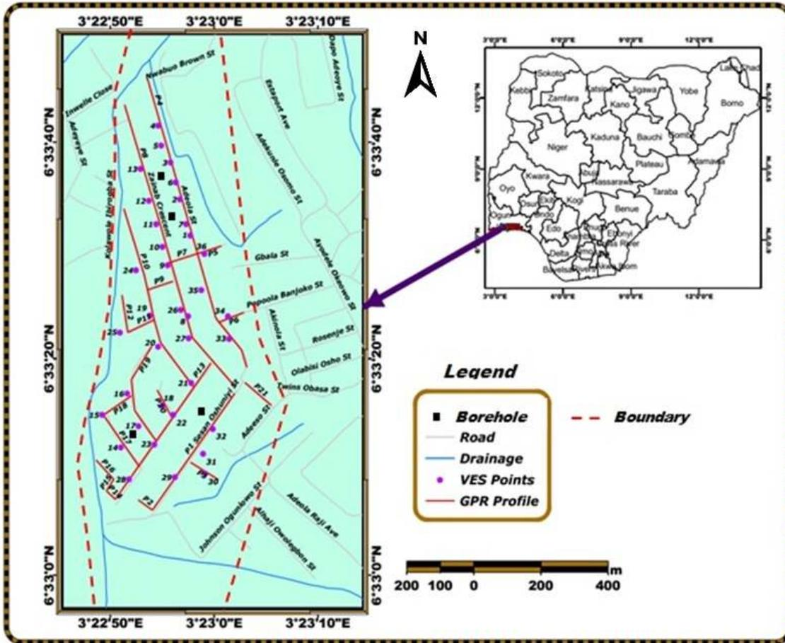
Figure 4: Field Layout of the study area showing the GPR profiles and VES points
