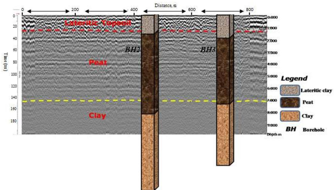
Figure 6b: GPR section of traverse 8 corroborated by borehole sections BH2 and BH3
