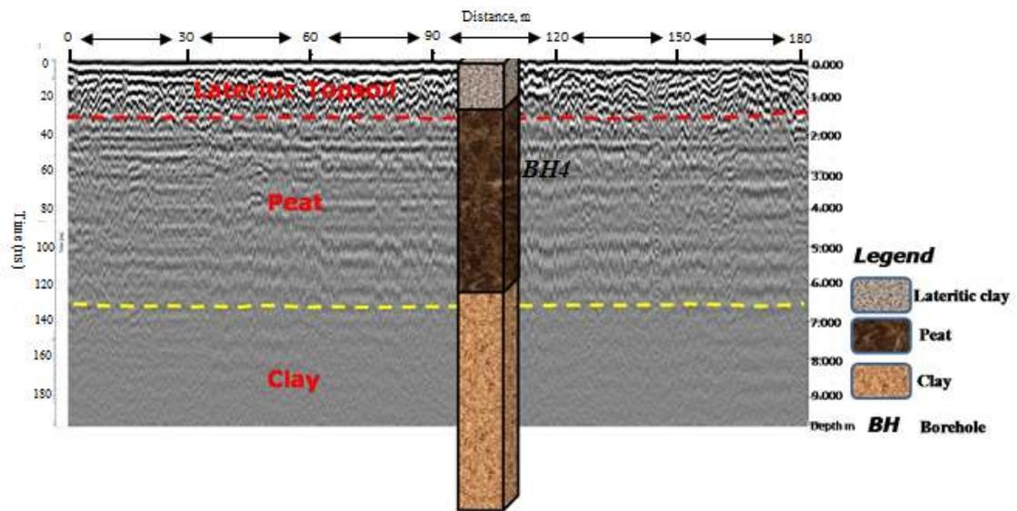
Figure 7b: GPR section of traverse 17 corroborated by borehole section BH4
