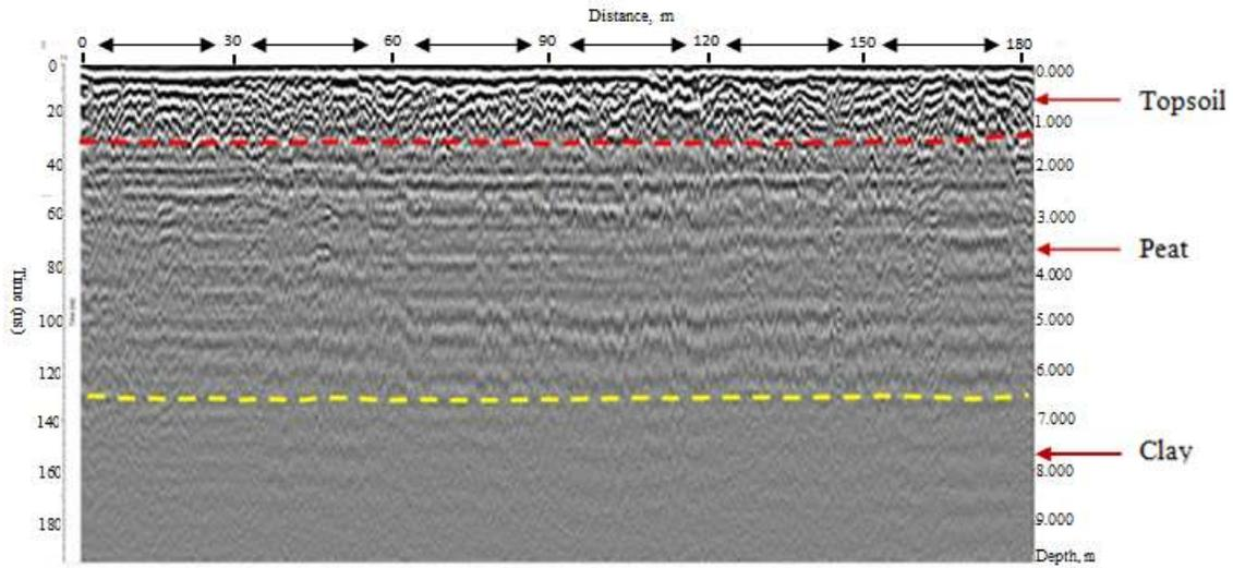
Figure 7a: GPR section of traverse 17
