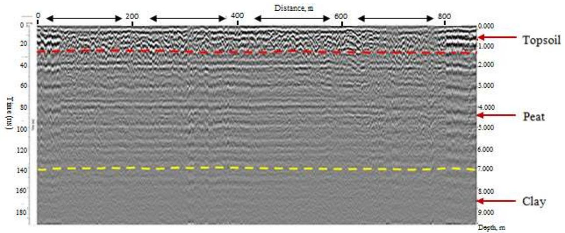
Figure 6a: GPR section of traverse 8
