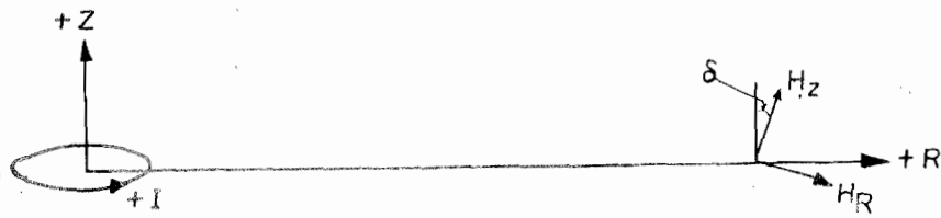
a) T_x - R_x Geometry and Misorientation Angle \delta
