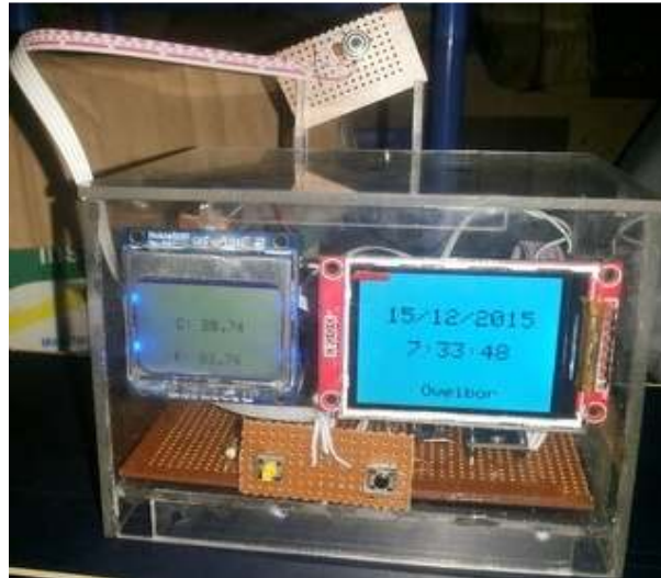
Figure 7: Constructed digital thermometer with clock
