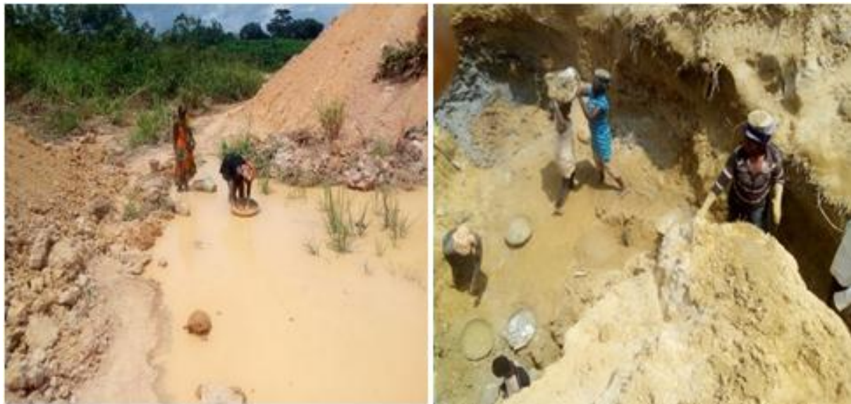
Figure 3. Panning (residual gathering method) and Load pottering (Semi-mechanised method –Chang-fa method) of females' engagement in galamsey
